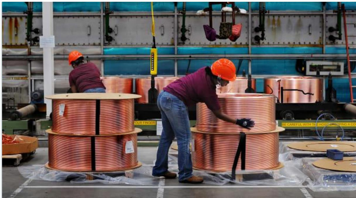
Factory workers secure large copper tube coils that will be wrapped and shipped out.
